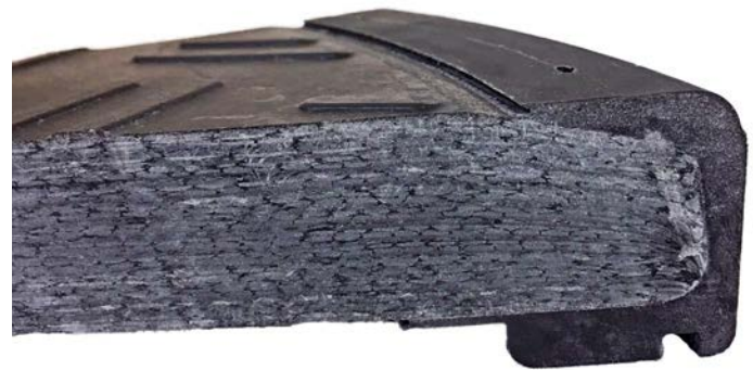
Cutaway showing the cover dampener around the outer edge (far right).
