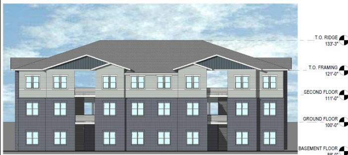
BUILDING 2 - REAR ELEVATION
