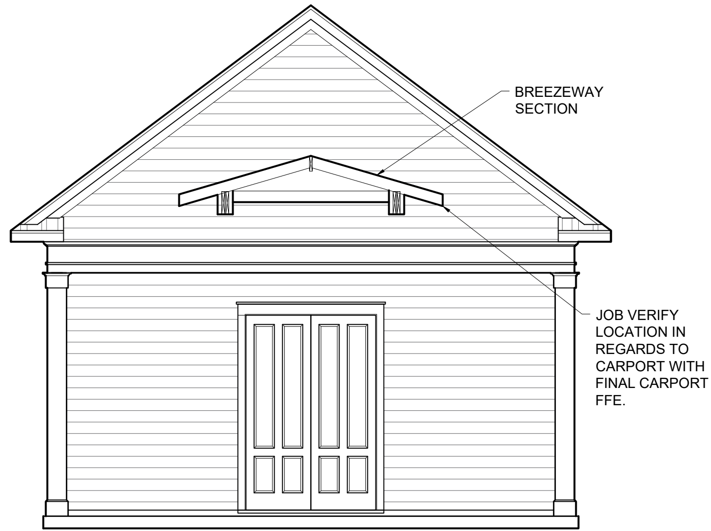
CARPORT LEFT ELEVATION SCALE: 1/4" = 1'-0"
