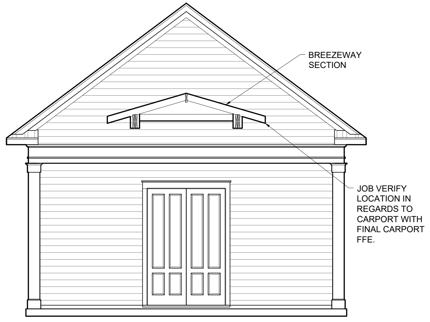
CARPORT LEFT ELEVATION SCALE: 1/4" = 1'-0"
