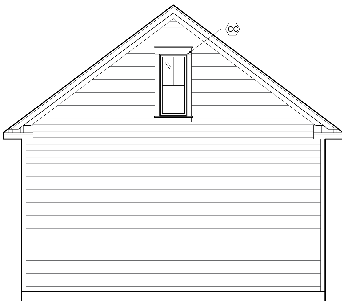
CARPORT RIGHT ELEVATION SCALE: 1/4" = 1'-0"
