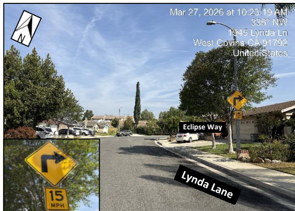
Curve Warning Sign & "15" MPH Advisory Speed along northbound Lynda Lane, approaching Eclipse Way.
