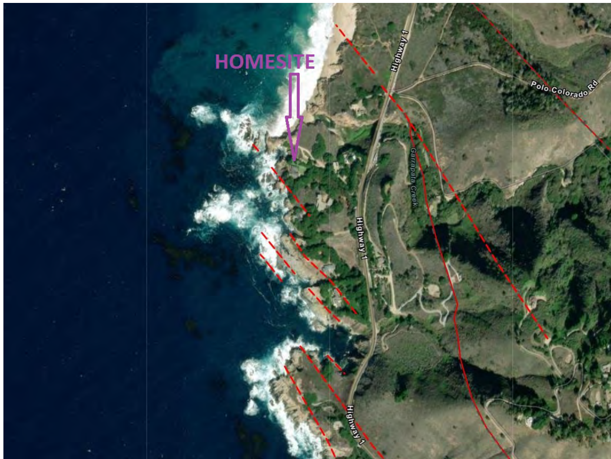
Figure 8: Close Up View of the Monterey County GIS Geologic Hazards Map Showing Mapped Fault Near Property
