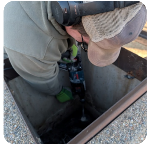
To prepare for precipitation from rain or snow and the upcoming busy season of park use, staff drilled additional holes in trashcans to allow for proper drainage.
