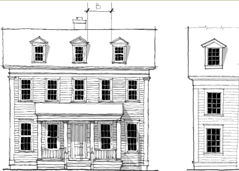
Dormer placement is based on the window pattern below, but does not repeat it. The distance between eaves is at least twice the width of the window.
