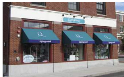
Vertical window proportions allow a traditional structural system with short spans and vertical piers to carry imposed loads to the ground.
