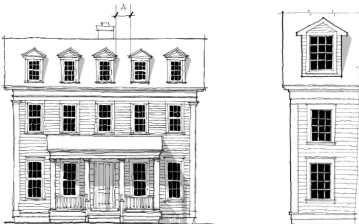
Avoid spacing dormers too closely with uncomfortably tight clearance at the eaves.
